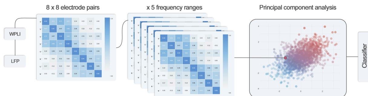
Figure 1 – Schematic diagram of mathematical analysis sequence of electrophysiological data
